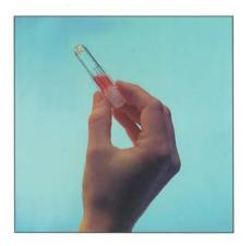
Take out the cuvette and mix vigorously (back and forth) to dissolve the reagent.
