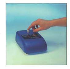
Blank measurement max. 40 seconds. Add the CRP-reagent by pressing down the inner part of the cap.
