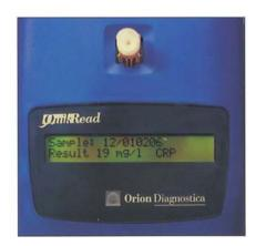
Put the cuvette back in the measurement well. Read the CRP result within 2 minutes.
